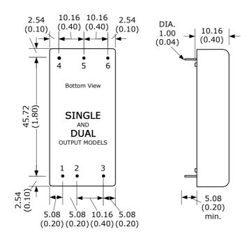
All dimensions are typical in millimeters (inches).
